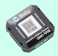
The UMD communicates with the UM8 Controller via the RS-485 Modbus RTU interface and can also be controlled directly through 2 digital input signals (impulse switches). The dimmer is suitable for both active and capacitive loads. The UMD has small form factor and can be installed behind lighting switches. Ideal for: Lighting automation and shading control
